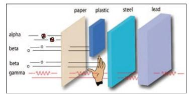
Fig. 2: Penetrating Power of Radiation [3, 4, 8, 10]
