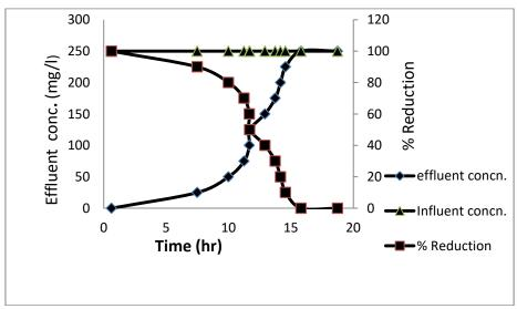
Figure-1: Dye Reduction at a bed height of 3cm for the activated carbon packed column
