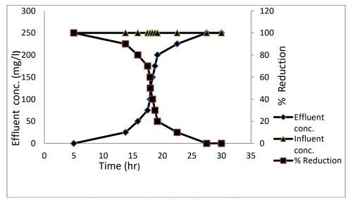
Figure-2: Dye Reduction at a bed height of 6cm for the activated carbon packed column
