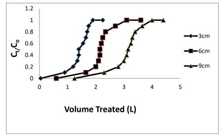
Figure-4: Effect of Bed Heights on packed Bed Column conditions; Co =250mg/l, flow rate =2ml/min, pH =7.5
