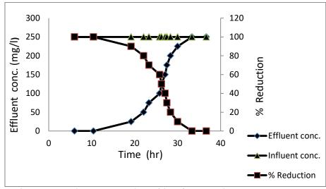
Figure-3: Dye Reduction at a bed height of 9cm for the activated carbon packed column
