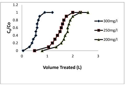
Figure-5: Effect of concentration on packed Bed Column conditions; Bed height =6cm, flow rate =2ml/min, pH =7.5
