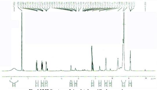
Fig- 4:NMR Spectrum of Acrylated epoxidized corn resin
