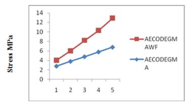
Percent Strain Fig-9: Stress and strain behaviour of the bio polyesters
