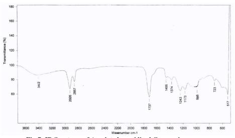
Fig-7: IR Spectrum of Acrylated epoxidized Corn resin
