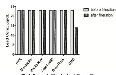
Fig-2: Removal of Lead using different filters
