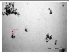
A. AL-AgNPs, nanoparticles showing spherical shape
