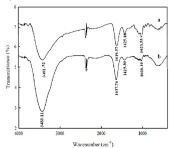
Fig: 3: FT-IR spectra of (a)Chitosan (b) Alginate
