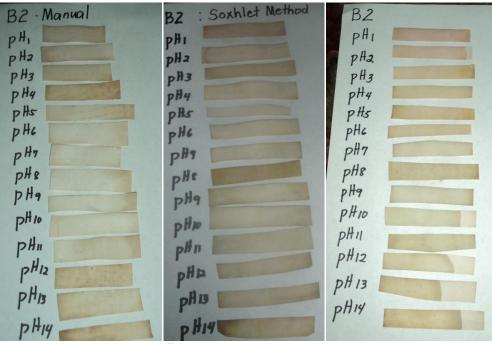
Manual MethodSoxhlet Method RotaryEvaporator MethodFig-2: Color reaction of Latundan (Manila)Bract Extract Paper Strips processed by the three (3) methods with<br/>solutions of varying pH.
