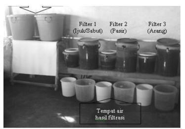
Fig- 1: Prototype equipment SPL Up flow
