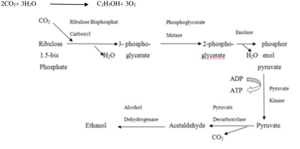
Figure 1. The production of ethanol through alcoholic fermentation (Emma and Rosalam, 2012).
