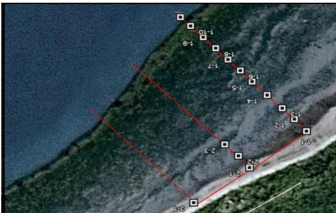
Fig-3: Illustration of the sampling device for a given site (in red: transects, 500 m apart from each other; in white: sampling points, 50 m apart along the same transect)
