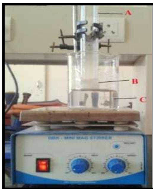
Fig-1: Laboratory designed diffusion cell (A- Tube containing formulation, B- Egg membrane, C- Beaker containing simulated tear fluid)
