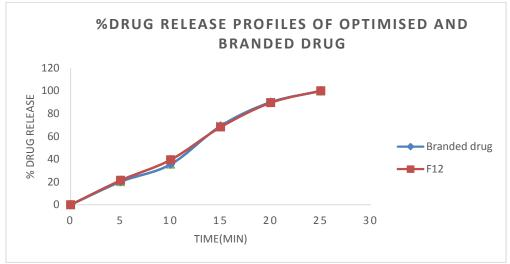
Fig 10: Dissolution graphs of Optimized formulation and Branded drug
