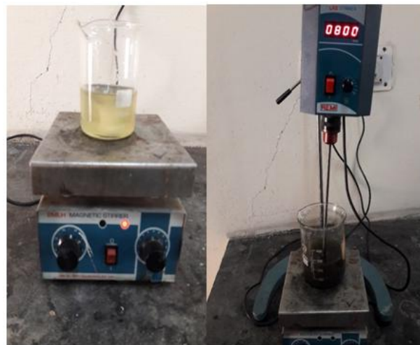
Fig-3: Magnetic stirrer and Mechanical shaker using to prepared suspension of drug polymer
