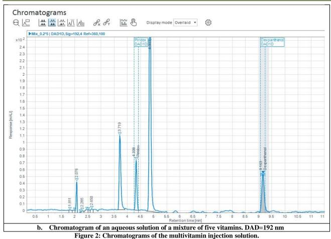
All five tested components are well separated. The slowest component, an isomer of Riboflavin 5'phosphate sodium, has a retention time of about 18 minutes so the run time was set to 30 minutes. UV spectra of the vitamins are presented in Figure 3, 4. Each
