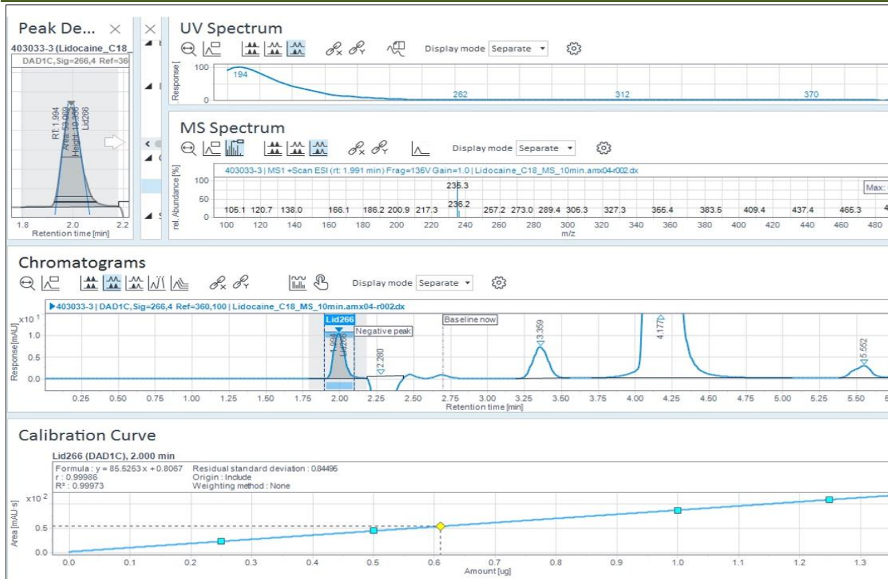
Figure 1: Lidocaine. Chromatograms, spectres, and calibration curves
