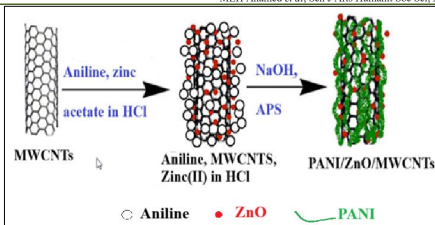
Figure 2: Preparation of PANI/ZnO/MWCNT by in-situ polymerization
