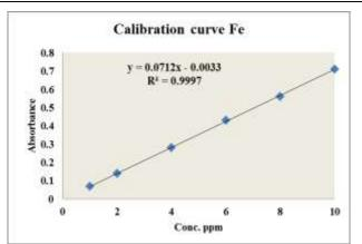
Fig -1: Calibration curves for the determination of Cu, Mg and Fe in the fruits and vegetables
