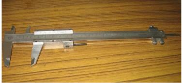
Fig-1: Vernier calipers of 0.2mms accuracy
