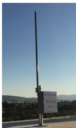
Fig-3: SkySens base station
