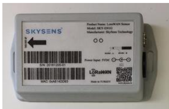
Fig-2: SkySens modem used for transmitting tractor performance data to base station
