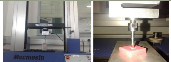
Figure 9: Fracture Resistance Test
