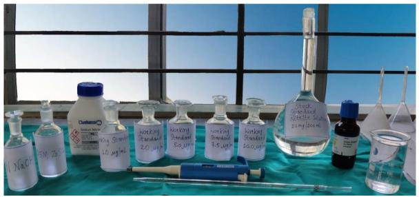
Figure 5: Preparation of Standard Nitrite Solutions at different concentrations
