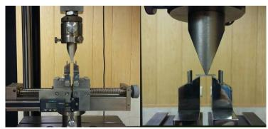
Fig-2: Universal testing machine for flexural strength test
