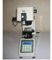
Fig-1: Vicker's microhardness tester
