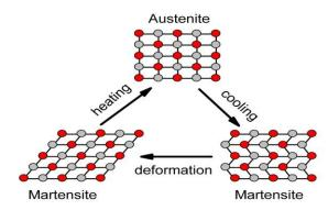
Diagrammatic representation of the shape memory effect of NiTi alloy Source:
