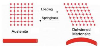
Diagrammatic representation of the superelasticity effect of NiTi alloy
