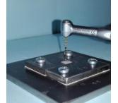
Fig-6: Using X-Smart plus Motor (300 rpm, 2.0 Ncm) to rotate the file until failure occur
