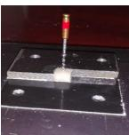
Fig-4: Side view of the file fixed in composite resin cube inside the custom made mold.
