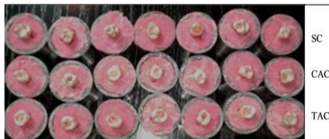
Fig-5: Maxillary Molars embedded in self-cure resin for Testing
