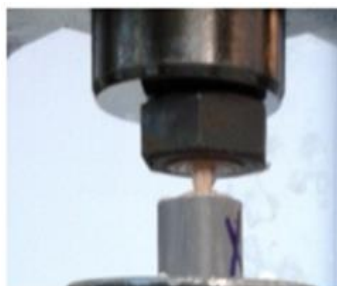
Fig-6: A sample tooth loaded for testing
