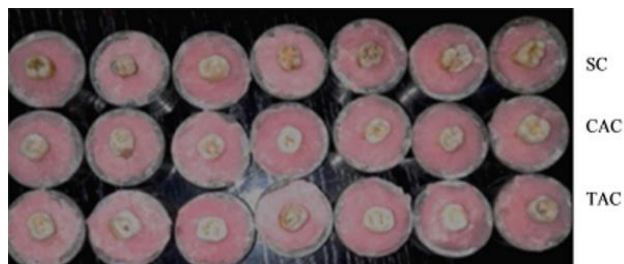
Fig-4: Mandibular Molars embedded in self-cure resin for Testing
