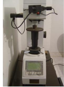
Fig. 11: Vickers Micro-hardness Tester
