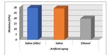
Figure 4: A column chart of total Young's Modulus mean values for different artificial aging
