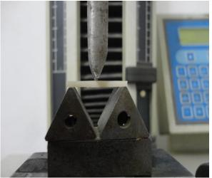
Fig. 8: The three point's test on universal testing machine
