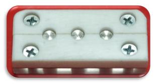
Fig. 9: Teflon mold 2×6mm diameter
