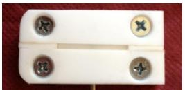
Fig. 6: Teflon mold 2×2×25 mm used for sample preparation
