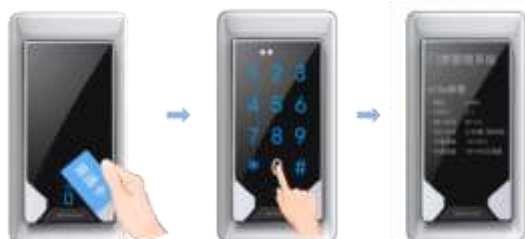
Fig-5: The Common Working Process Of IAMS
