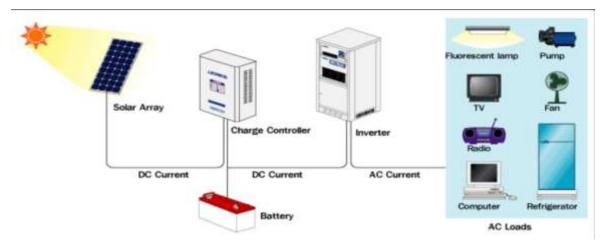
Fig-2: Solar electric power system layout
