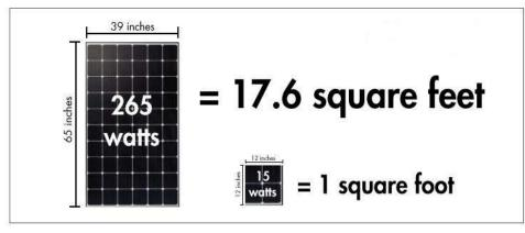
Fig-1: Area requirement for Solar PV installation
