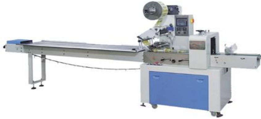
Figure 10: Multi-function automatic pouch packing (Source: Writing Team, 2022)
