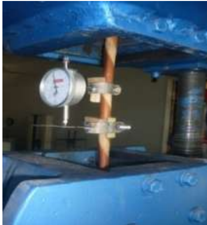
Figure 1: Tension Testing of Rattan in UTM
