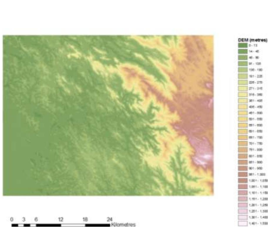
Figure-2 :DEM Used For Watershed Delineation
