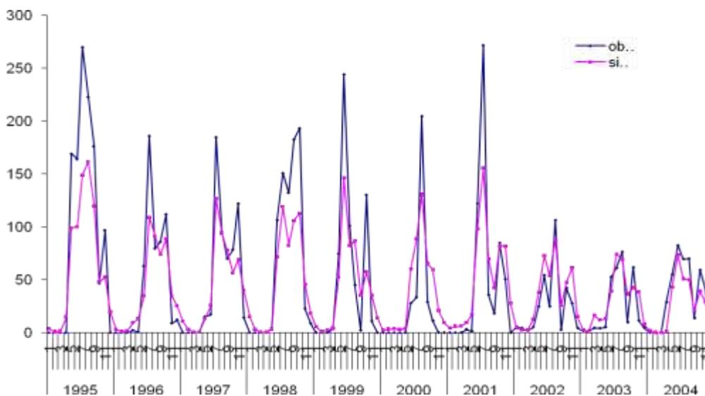
**Figure 7 Observed and simulated streamflow at Peroor for the validation period.**
