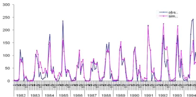
**Figure 6 Observed and simulated streamflow at Peroor for the calibration period.**
