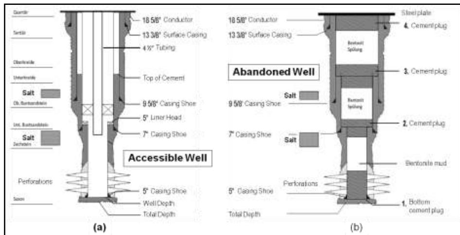
Fig. 1: (a) Accessible well structure (b) Abandonment standard (Reinicke and Fichter [1])
