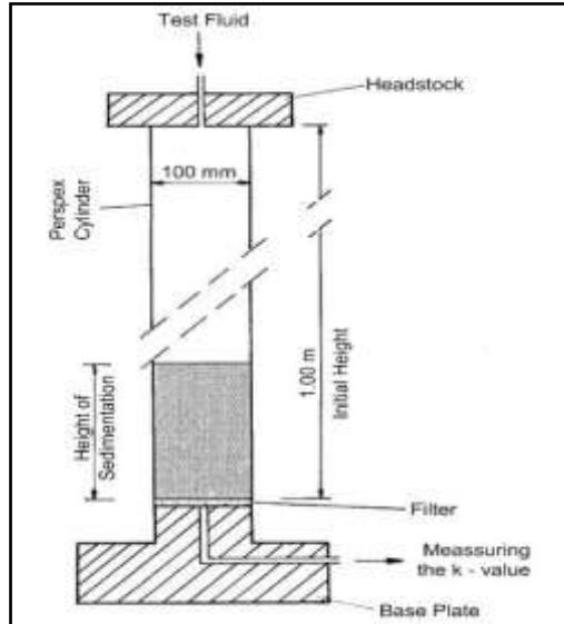
Fig. 5: Schacht Konrad test unit (Wittke [25])
