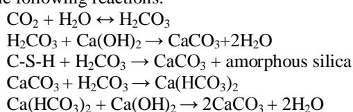
The calcium carbonate continues to react with the carbonic acid and builds water-soluble calcium bicarbonate. The last reaction is very critical, because the formation of water allows dissolution of more CO<sub>2</sub> [3, 4].
