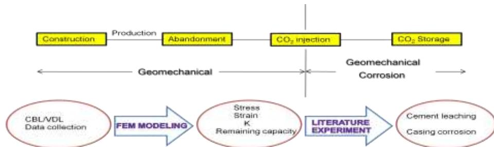
**Fig. 6: Process affecting well integrity in the well life**
