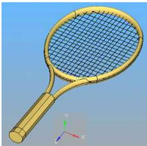
Figure 1a: 3D Model of the tennis racket
