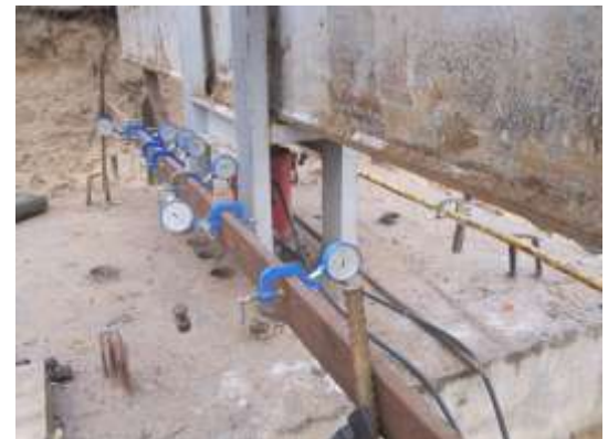
Fig. 4: Dial gauges for Settlement Reading
