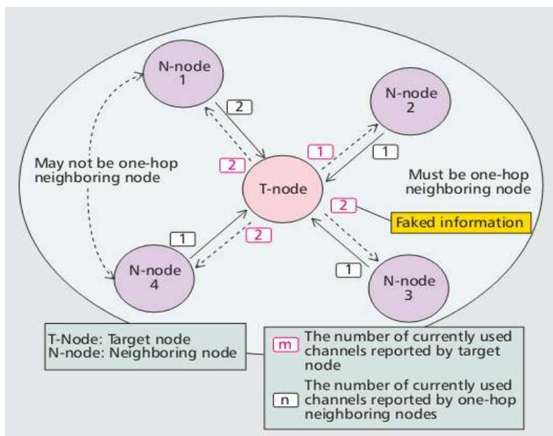
**Fig. 1: Detection mechanism for selfish attack**
