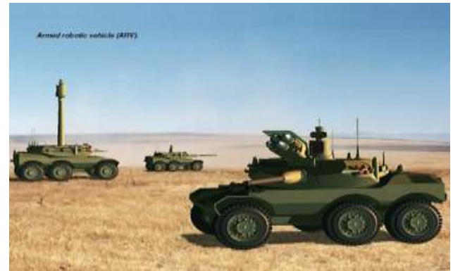
Fig- 2: Armed Robotic Vehicle (with communication relay and anti-tank weapon mounted)
