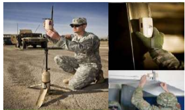
Fig-7: Tactical Unattended Ground Sensor
