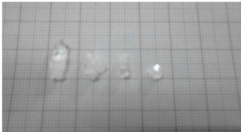
Fig-2: Crystal grown in gel Zn doped KHC_4H_4O_6
