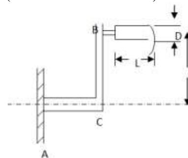
**Fig. 1: Design recommendation for crank handle.**
