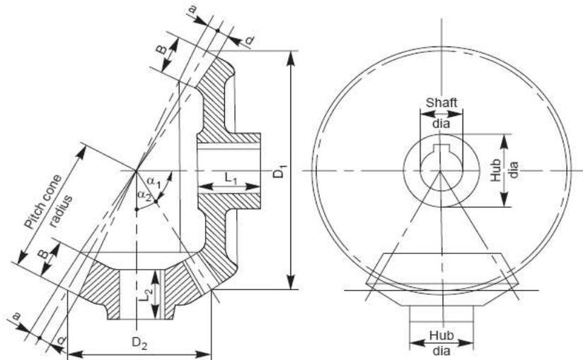
Fig- 2: Bevel gearing
