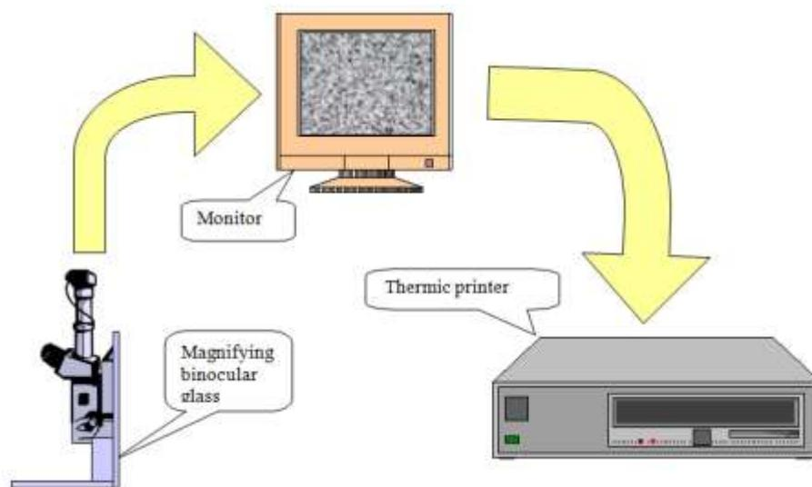
**Fig-2(A): The device of image acquisition**
