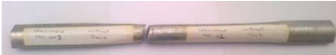
Fig- 3: Broken pipe specimen
