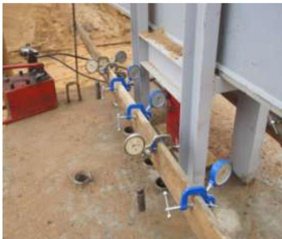
Fig.5: Dial gauges for Settlement Reading
