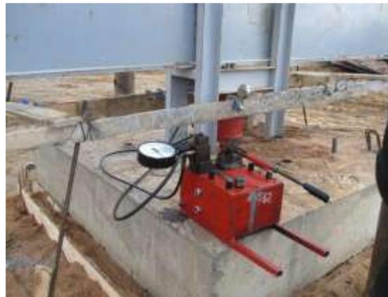
Fig.4: Loading device of 200T capacity HJ
