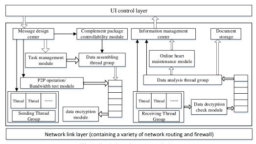
Fig-1: Real-time data transmission
