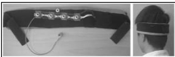
(g) Fig-8: An EEG headband with an embedded data acquisition and wireless telemetry unit [81].
