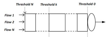
Fig- 1: Threshold Dropping Queue with N Drop Precedence
