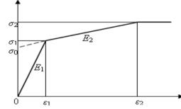
Fig-3: Three line model for stress-strain relations
