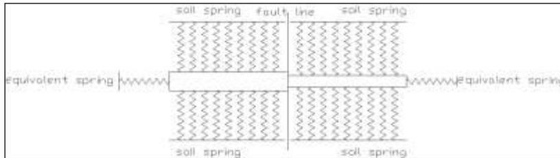
Fig-2: Schematic diagram of buried variable-diameter pipeline across the fault
