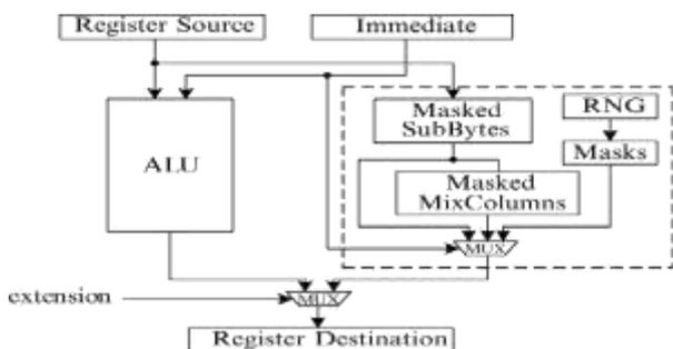
Fig. 7 Structure of the proposed extension in the AES-M1 design
