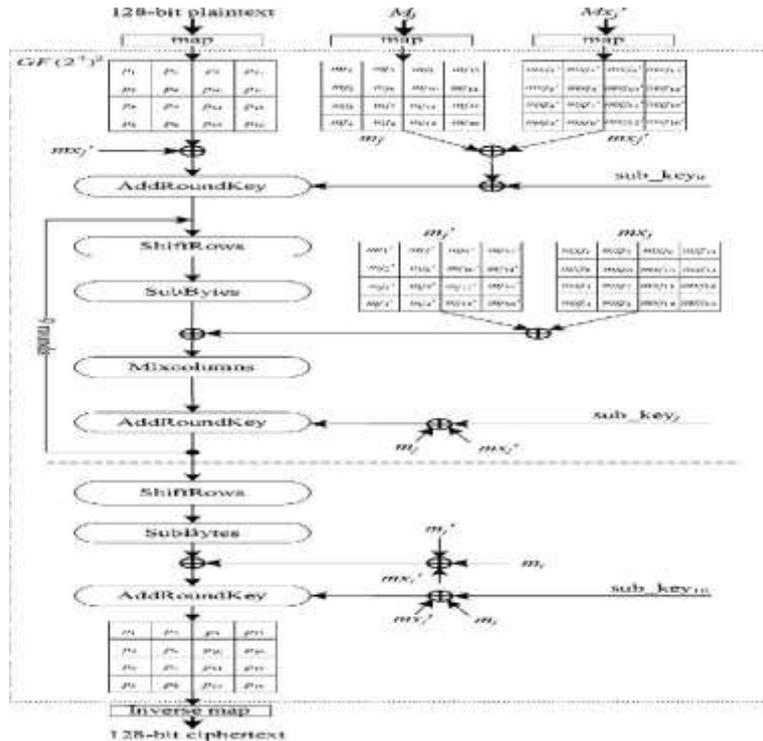
Fig. 6 Structure of the proposed first-order masked AES design
