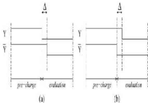
Fig. 3 Time domain data encoding (A) Logic '1'; (B) Logic '0'
