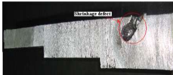
Fig-7: Section of casting with shrinkage defect
