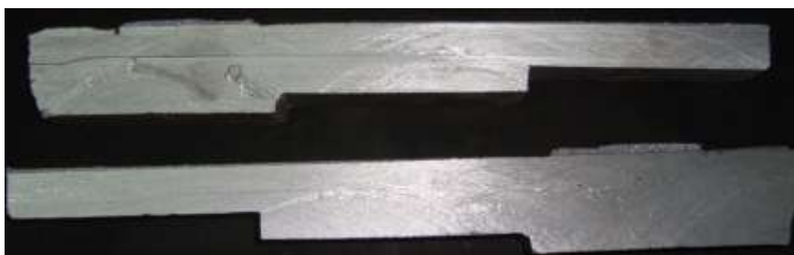
Fig-28: Section of casting shows no shrinkage defect
