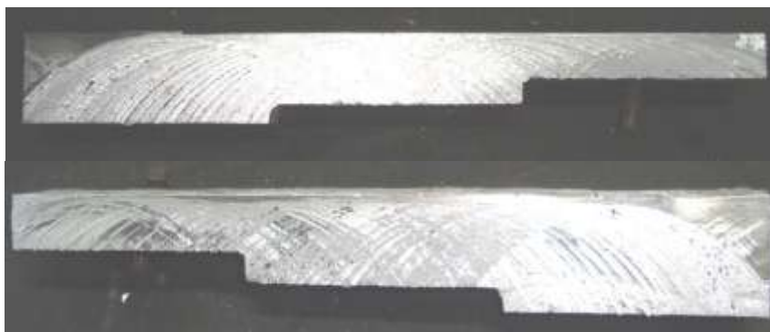
Fig-14: Section of casting shows no shrinkage defect
