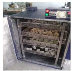
Fig-2: Arrangement of food samples in the dry
