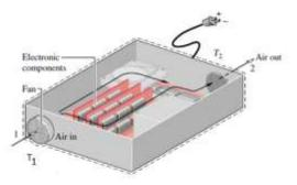
Fig.2 cooling of electronic components
