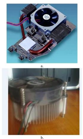
**Fig-1.0:** Blower-heat sink system for an electronic appliance.
